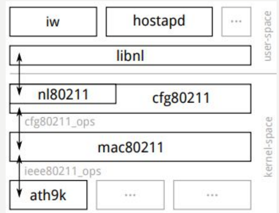
Fig. IEEE 802.11 Linux kernel implementation architecture
