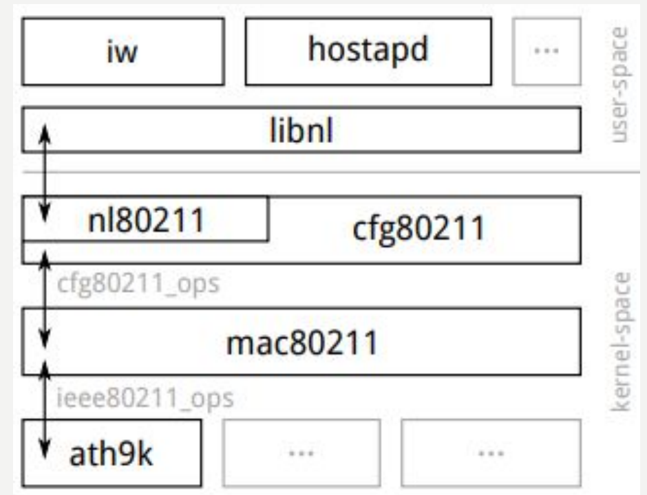
Fig. IEEE 802.11 Linux kernel implementation architecture
